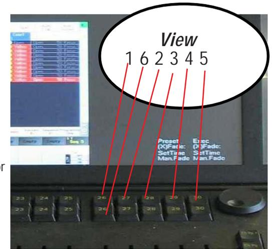
To empty a screen press V4 und V9 simultaneously (right monitor) or press buttons 11/11 or 26/26 (picture above) simultaneously for center and left monitor)
