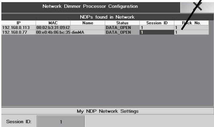
IP: The IP network addresses of the devices
