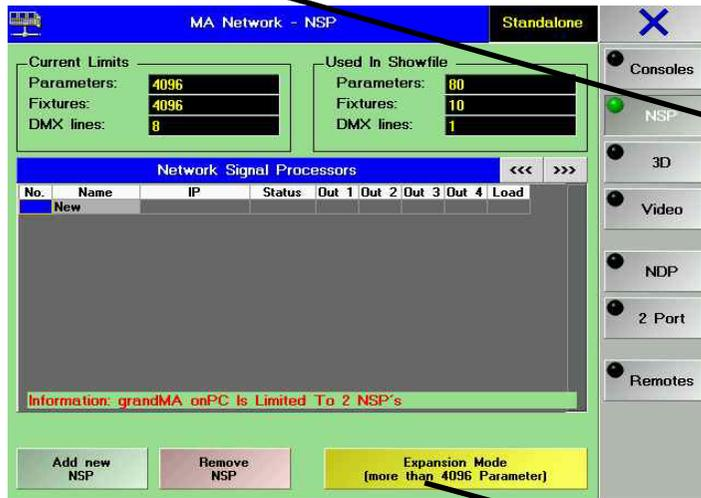
**LOAD** columns (numbers 0 - 100). Will show the workload of the data output of the respective NSP. If the number in this column is displayed in red, the NSP is temporarily overloaded. This will somehow decrease the normal DMX repeat rate of approx. 30 Hz. This can be disturbing e.g. with moving lamps or stroboscopes.
