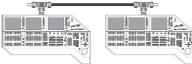
Two *grandMA* consoles connected on a 10 Base-2 network
