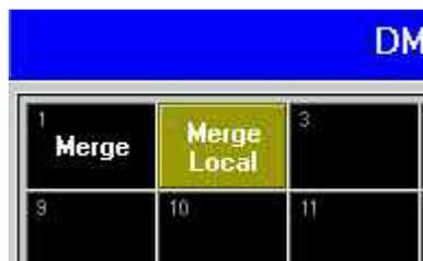
By pressing a button in the CONFIGURATION column you can call up the respective menu for this DMX output.
