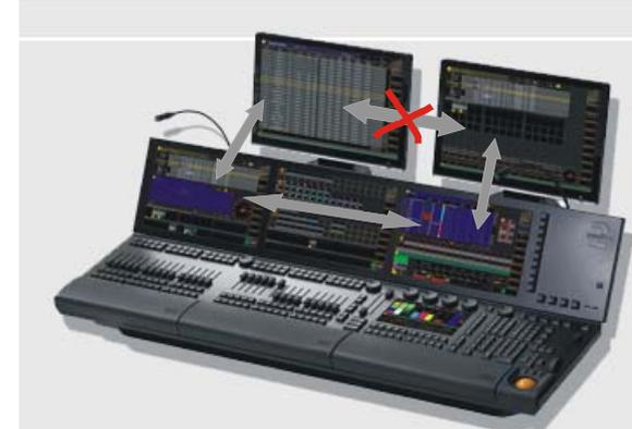
**Full-size:** leave the left and right monitor on the top side to enter the external monitor
