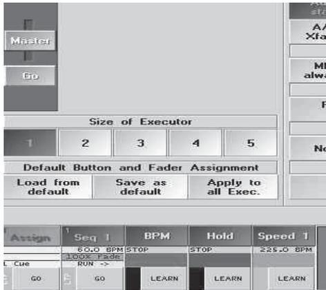
Micro - Assignment Menu; only one button and the fader (1-5, depends on size of executor) can assigned here.
