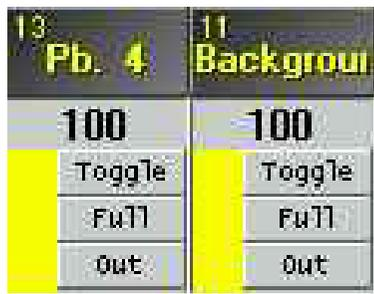
**Toggle:** When engaged, it will switch over from Full to Out and vice versa
