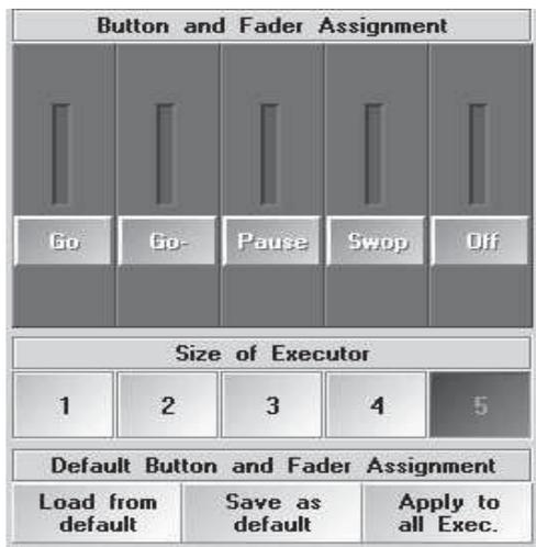
Assignment Menu of a fader button: only the button (1-5, depends on size of executor) can assigned here.
