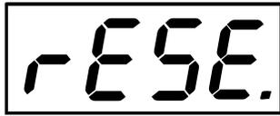
Press **[Enter]** button to run a reset. This option enables the WASH 575 XT to index all effects (functions) and return to their standard positions.
