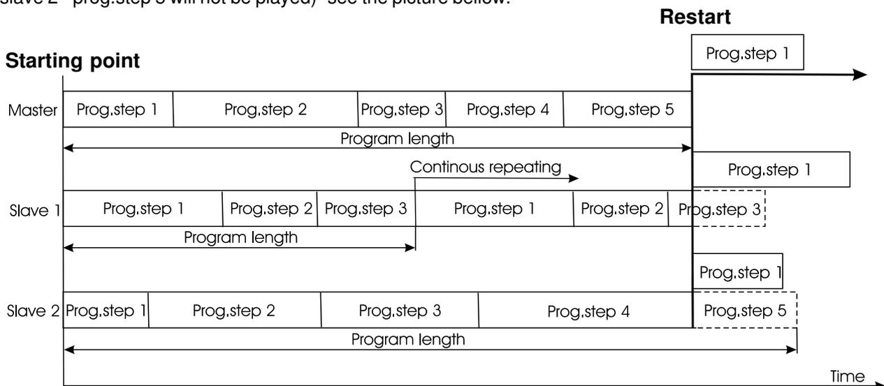
**Note:** Disconnect the fixtures from the DMX controller before master/slave operating , otherwise data collisions can occur and the fixtures will not work properly!
